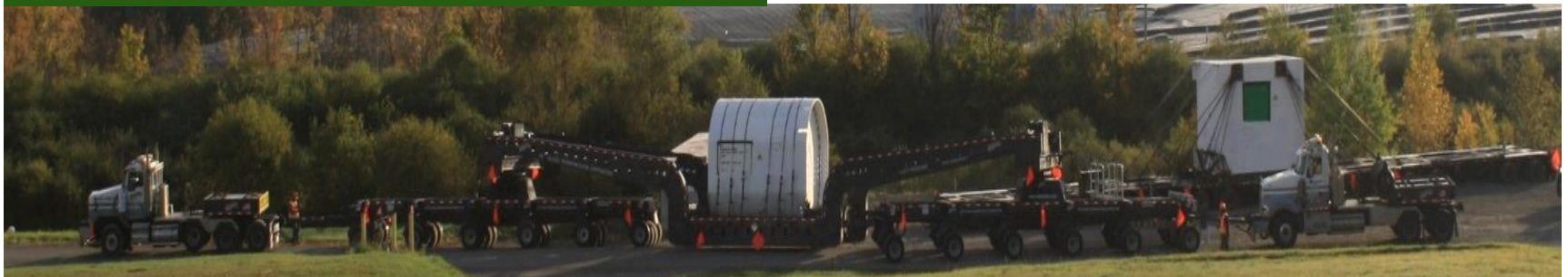
Heavy haul truck/trailer used to transport waste containers from WVDP.
